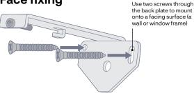
The bracket for face fixing should be attached using two screws through the back plate (side without the attaching bracket) onto facing surface such as wall or window frame.
