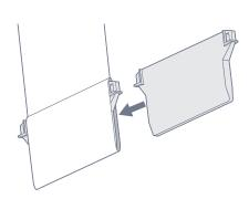
Slide the weight into the pocket at the bottom of the louvre.
