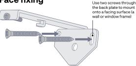
The bracket for face fixing should be attached using two screws through the back plate (side without the attaching bracket) onto facing surface such as wall or window frame.
