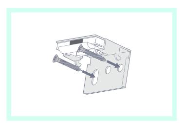
The outermost brackets should be mounted at least 5cm in from the ends of the blind.
